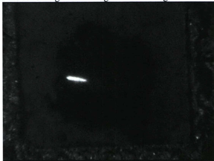
Figure 55. Filament = 24V(boost), G1 = -0.7V G2 = 438V, G3/5 = 5.0kV, G4 = -226V, G6 = 2.2kV, Target = 5.74kV, Target current = 900uA.
