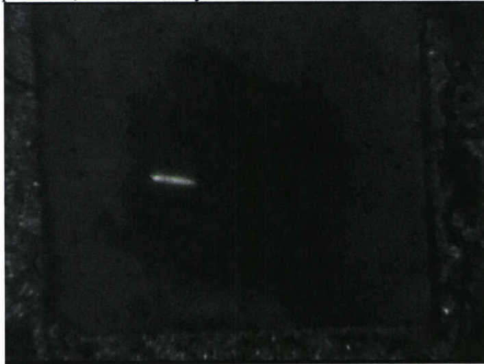
Figure 54. Filament = 24V(boost), G1 = -0.7V G2 = 325V, G3/5 = 5.0kV, G4 = -226V, G6 = 2.2kV, Target = 5.74kV, Target current = 600uA
