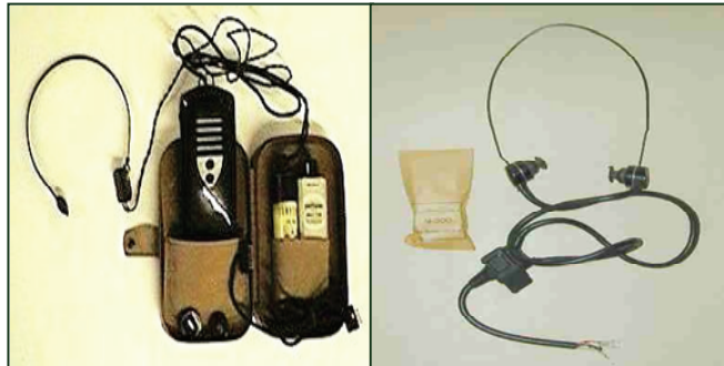
Figure 2. Sonotone's B-533 bone conduction body hearing aid (left) and M-300 system developed for the U.S. Signal Corps (right). (Pictures courtesy of Sonotone, Inc.)
