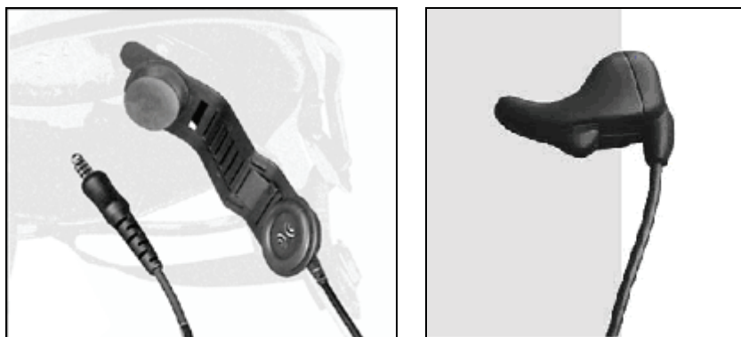
Figure 72. Two hybrid bone conduction communication devices from Savox Communications. (The left panel shows the HS-C and the right panel shows the EC. Both have a bone conduction microphone and an air conduction loudspeaker. The HS-C is designed to be mounted in a helmet and the EC is worn in the ear canal. Downloaded from: http://www.savox.com , October 6, 2006.)
