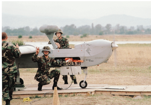
Figure 9. A U.S. Army Hunter UAV Is Prepared For Launch
