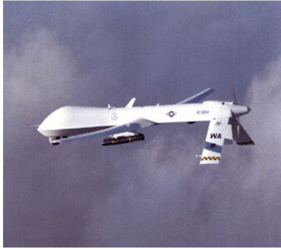
Figure 7. Predator Flying in Support of OEF, Equipped with Hellfire Missile
