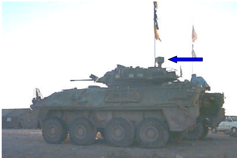
Figure 4: DAS Phase I prototype installed on a Coyote LAV.
