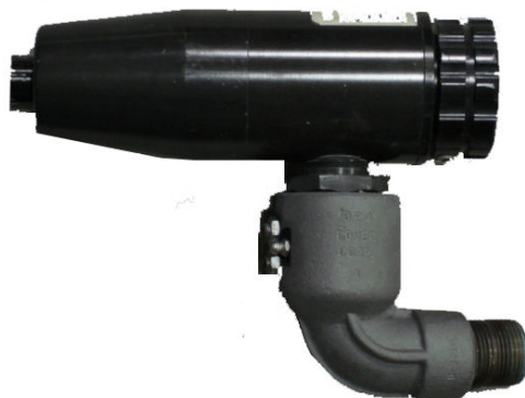
Figure 4.3.3: UHP P-19 tested 300 gpm combined agent Williams Hydro-Chem™ bumper turret nozzle.
