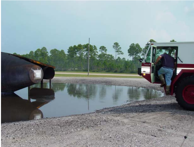
Figure 4.8.2: Preparation for a preliminary pressure impact measurement with a UHP bumper turret nozzle.
