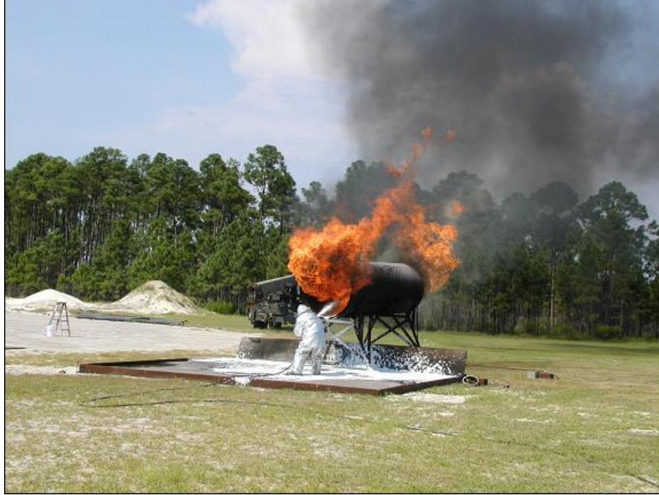
Figure 2.1.4: UHP attacking a 4 gpm continuously running fuel fire from an engine nacelle.
