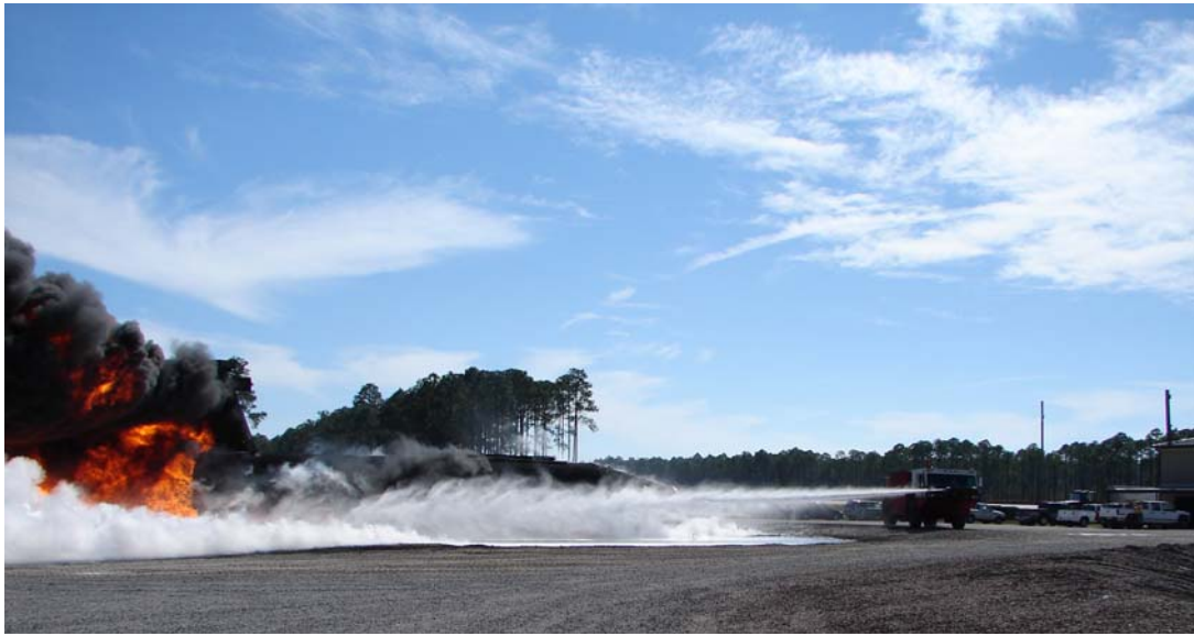
Figure 4.6.5: The UHP P-19 extinguishing a 3500 foot JP-8 fuel fire using UHP bumper turret nozzle #2.
