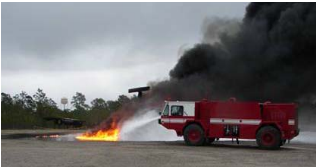
Figure 4.6.4: The UHP P-19 extinguishing a 3500 foot JP-8 fuel fire using UHP bumper turret nozzle #1.
