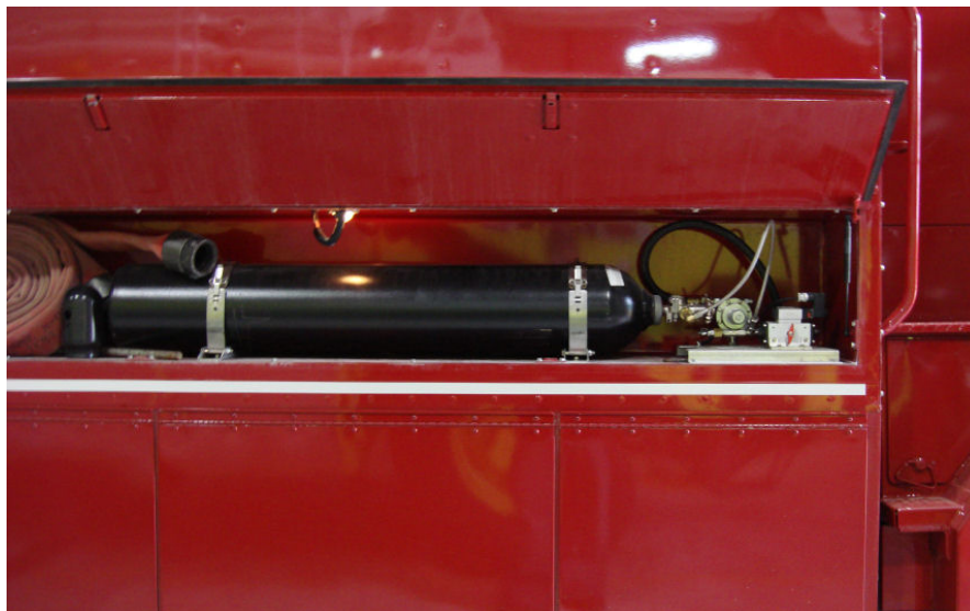
Figure 3.6.2: The high pressure nitrogen tank used to pressurize the dry chemical storage tank.
