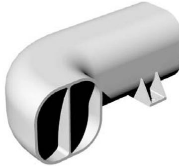
Figure 3.5. Rapid manufacturing design: An example of reducing part count from 16 parts to 1 part. (Courtesy, Loughborough University Rapid Manufacturing Research Group)
