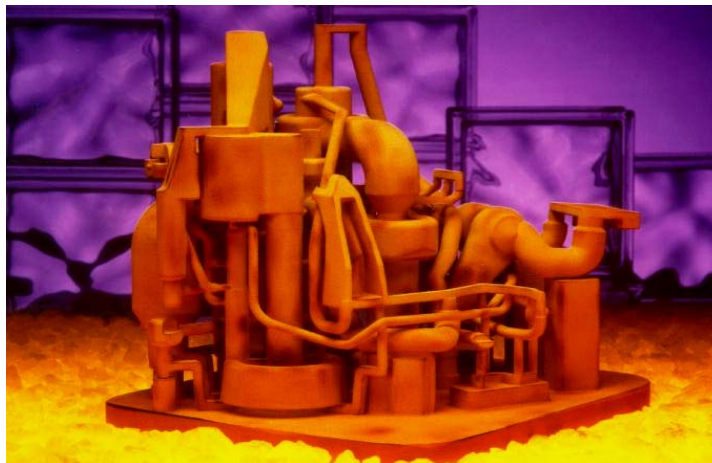
Figure 1.2. Complex SFF part created in a selective laser sintering process. (Courtesy 3D Systems)
