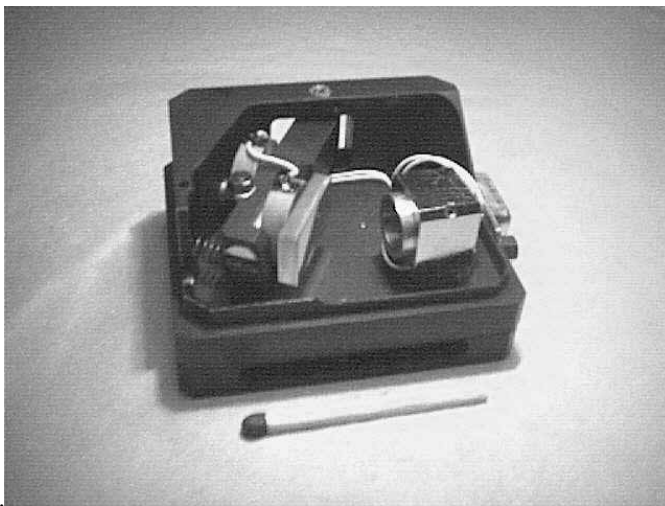
Fig. 9. The master laser (extended cavity diode laser).
