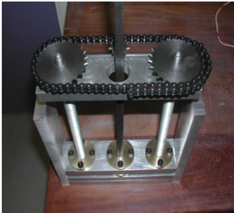
Figure 6. Manufactured Adaptive Stiffness Torsion Bar Concept.
