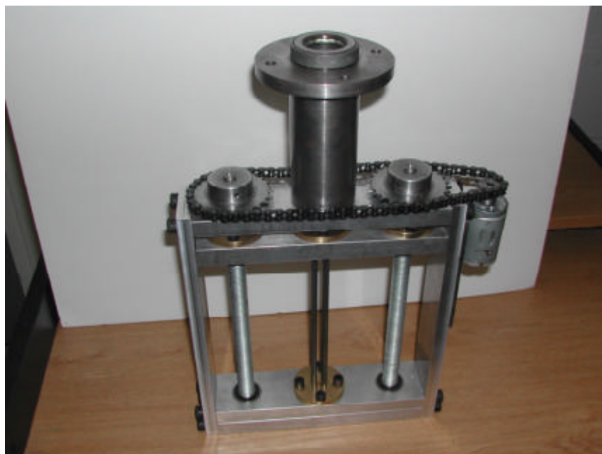
Figure 7. Manufactured Adaptive Stiffness Four Rods Concept.
