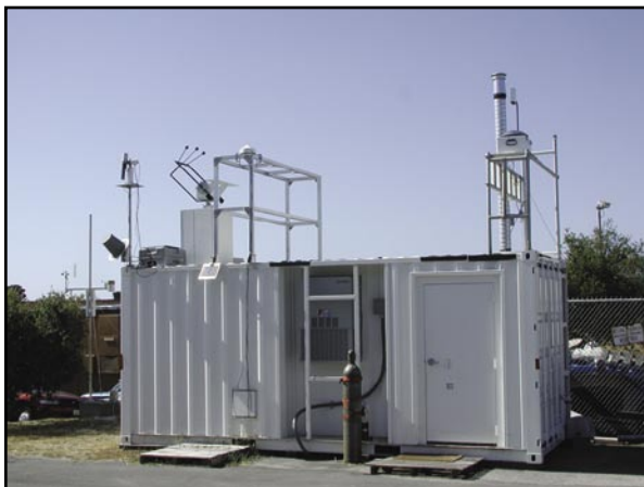
The Mobile Atmospheric Aerosol and Radiation Characterization Observatory (MAARCO) can be deployed in areas with limited facilities, even onboard ship, to gather data to support research on atmospheric aerosols, gases, and radiation. In August 2004, MAARCO was used in a field experiment in the United Arab Emirates.
