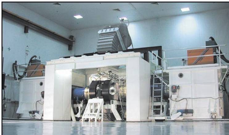
The NRL Electra system is used to develop high-energy high-repetition-rate KrF laser technology. The Electra 30-cm aperture electron-beam-pumped amplifier is shown in the photograph. A portion of the recirculating system that cools the laser gas can be seen at the top. This amplifier is capable of a 5 Hz repetition rate and is expected to produce more than 500 J of laser light per pulse.
