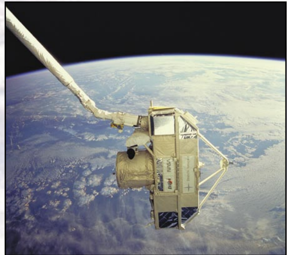
The German SPAS pallet was released from the Space Shuttle to operate as a free flying satellite for a week, then returned to the Shuttle. The SPAS contained a number of instruments to study the upper atmosphere, including NRL's MAHRSI, a high-resolution ultraviolet telescope.
