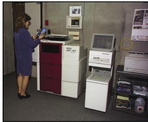
Technical Information Services' new Noritsu digital minilab can produce low-cost photographic prints, ranging in size up to 12 x 18 inches.
