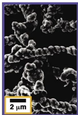
Metallic Cu spiral/helical nanostructures prepared via selective electroless metalization of a phospholipid microtubule template.
