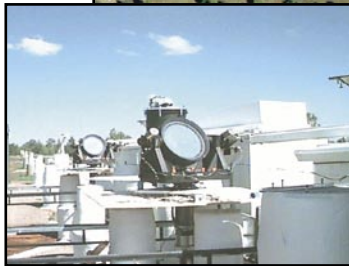
The Navy Prototype Optical Interferometer (NPOI) is used for both operational astrometry and for development of distributed aperture imaging techniques.
