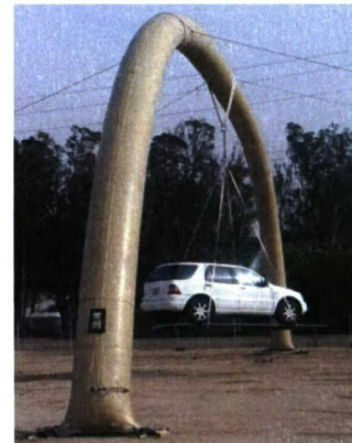
Fig 1. Inflated fabric arches used in aircraft shelters (left); Demonstration of arch load-carrying capability (right).
