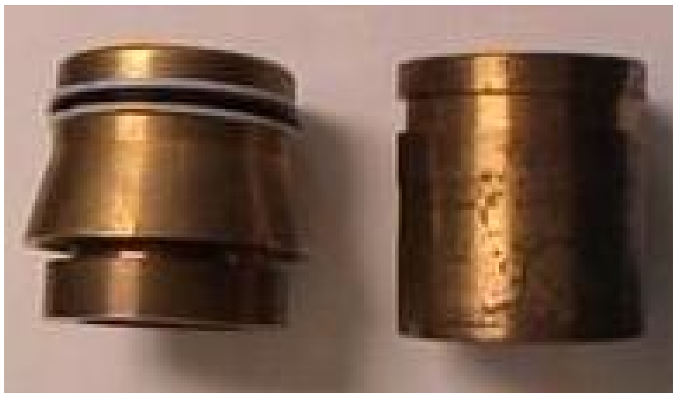
Figure 1 Left - Projectile skirt prior to firing. Right – skirt folded after firing.
