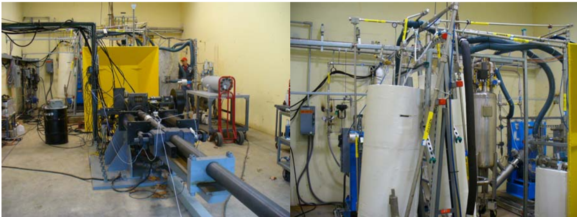
Figure 5 – (Left), 45mm CLGG with cryogenic feed system installed. Note that this system is oversized to feed the 155mm CLGG also. Right view shows closer view of accumulators (foreground) and pumps (background).
