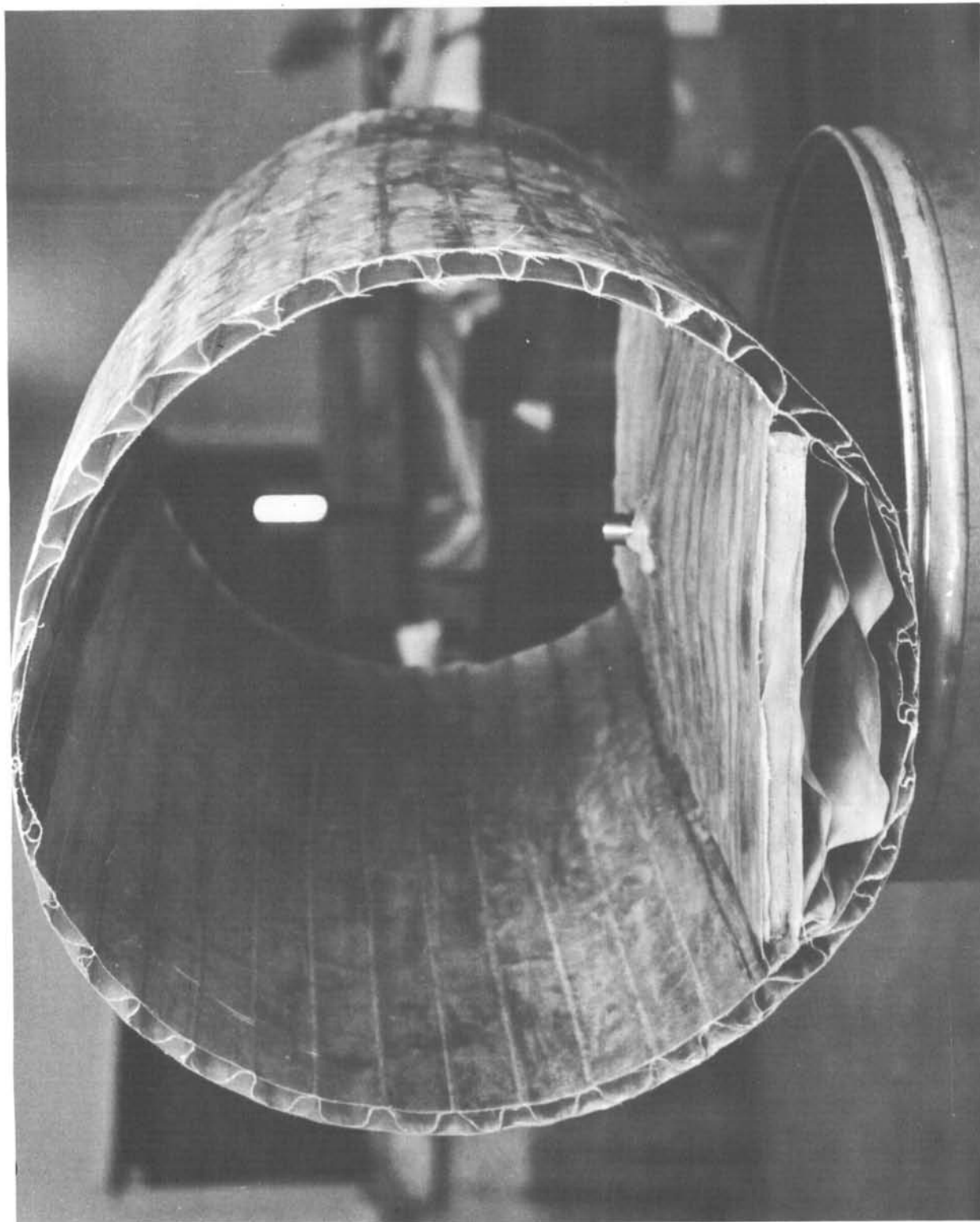
FIGURE 15 - CYLINDER WALLS IN 1/6 SIZE CYLINDRICAL SPACE STRUCTURE
