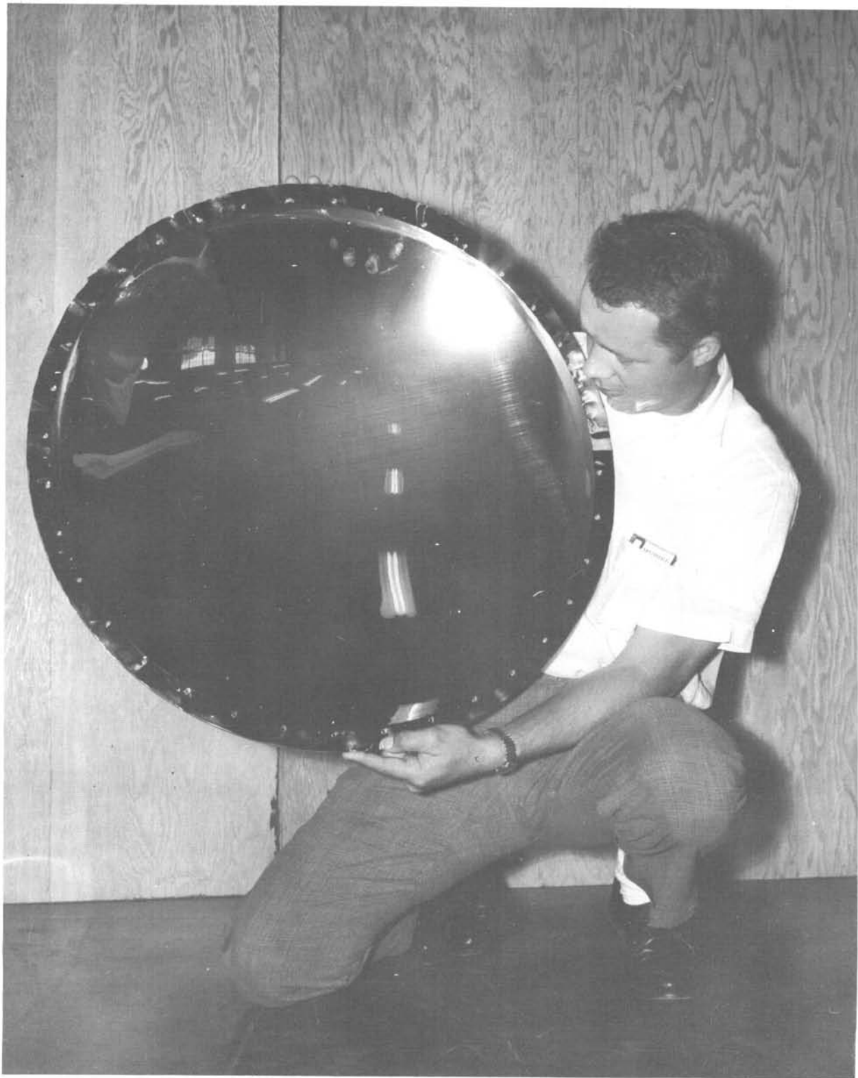
FIGURE 4 - VACUUM CURED 2 FT SOLAR COLLECTOR MODEL
