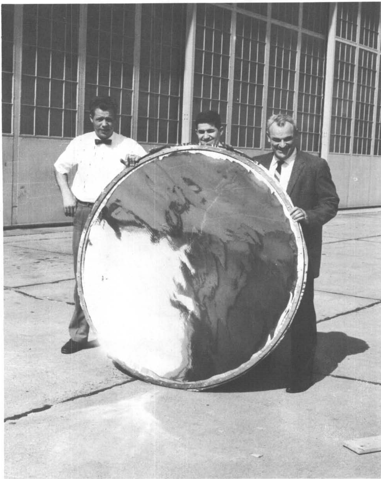
FIGURE 5 - VACUUM CURED 5 FT DIAMETER SOLAR COLLECTOR MODEL
