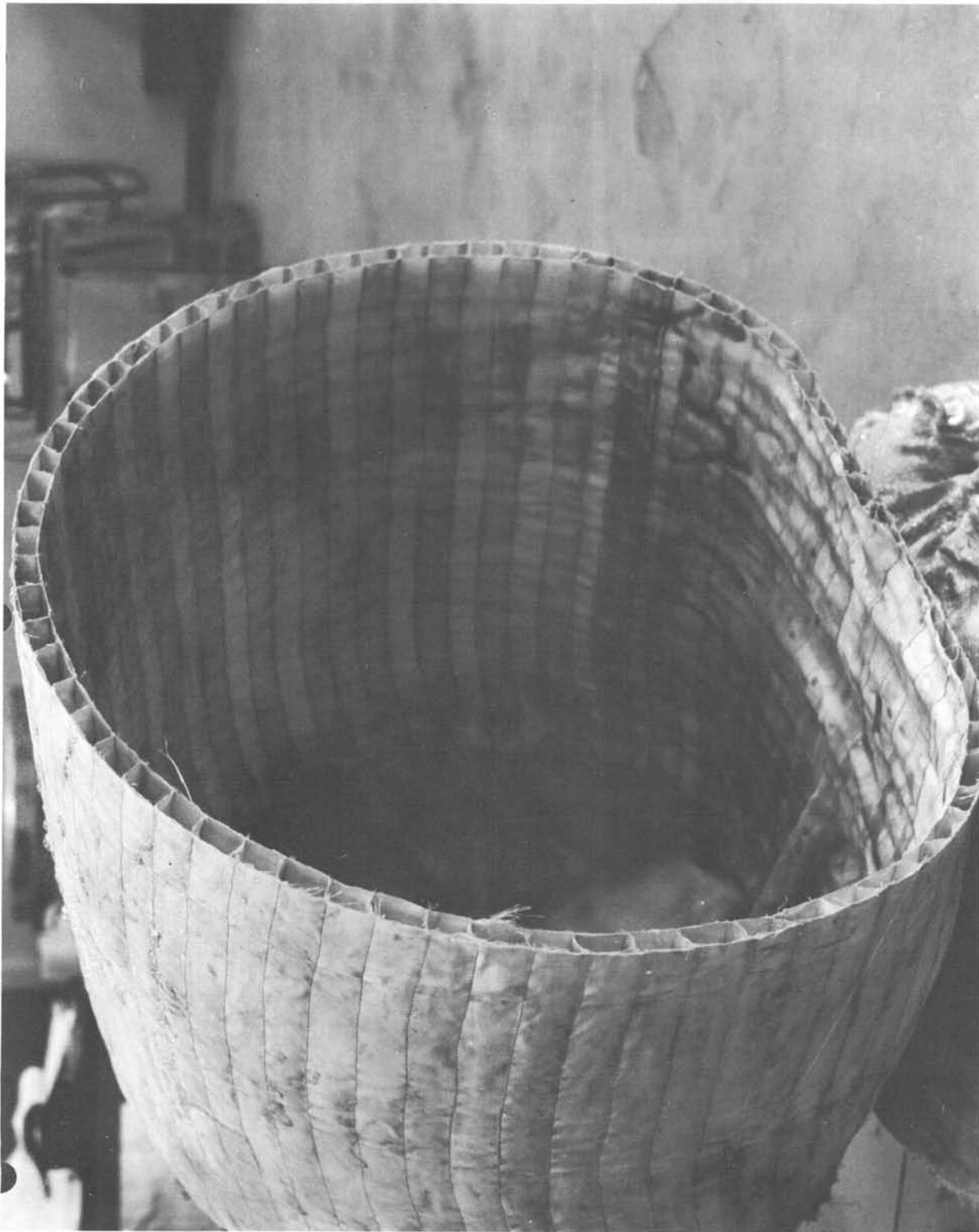
FIGURE 8 - GELATIN CURED 3 FT DIAMETER CYLINDER
