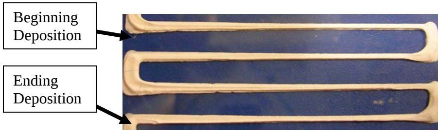
Figure 2: Deposition lines using constant ram velocity ( v = 0.5 \mu m/s ).
