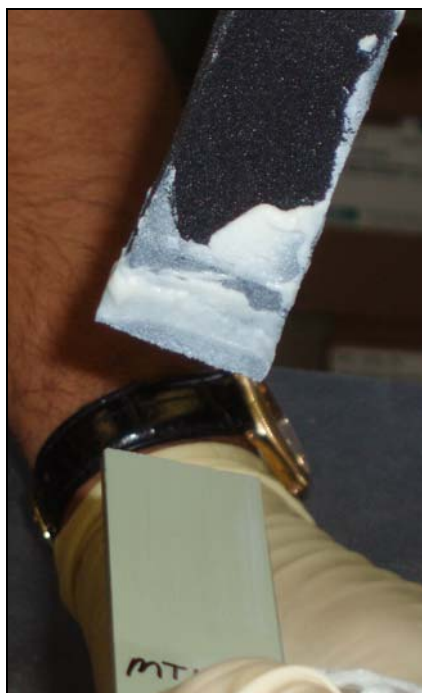
Figure 6. Foam brush filled with SILC prior to application of the coating to the coupon surface.
