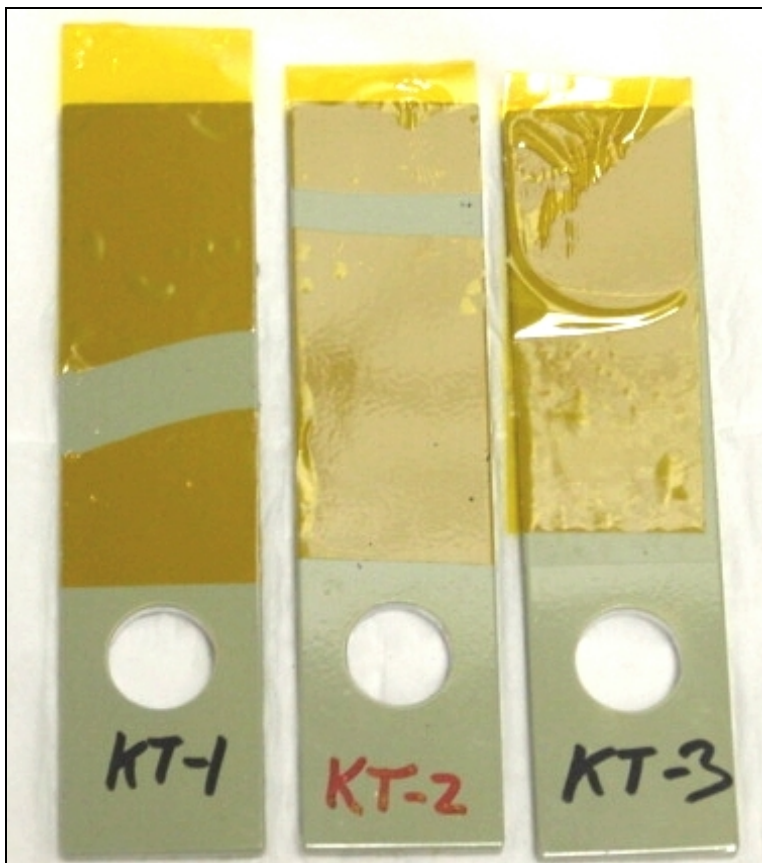
Figure 18. Failed Kapton tape and adhesive resulting from uncoated DLS testing.
