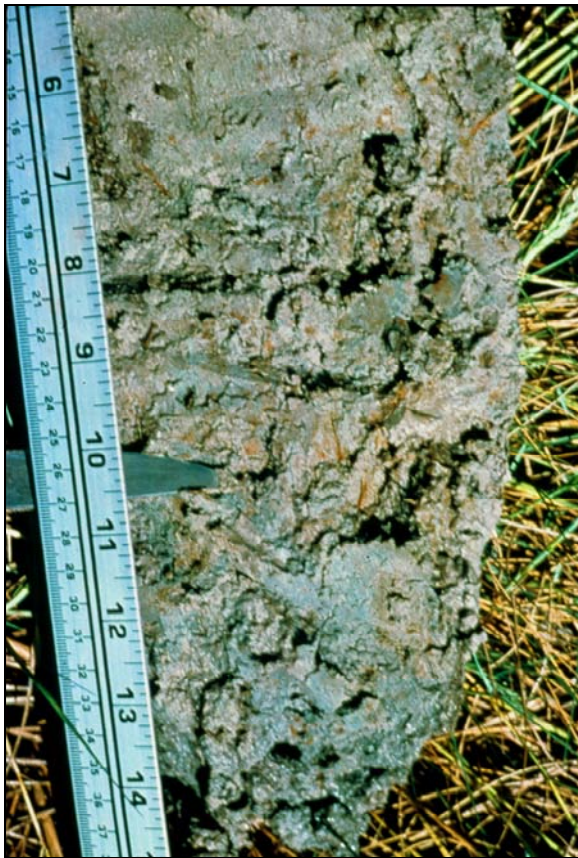
Figure 15. Indicator F3, Depleted Matrix. Redox concentrations are present within a low-chroma matrix.
