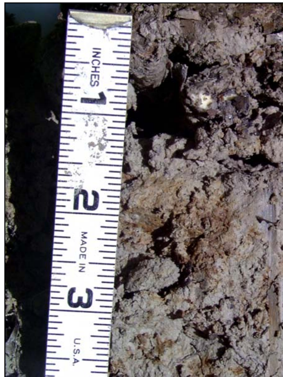
Figure 16. Redox concentrations at 2 in. (5 cm).
