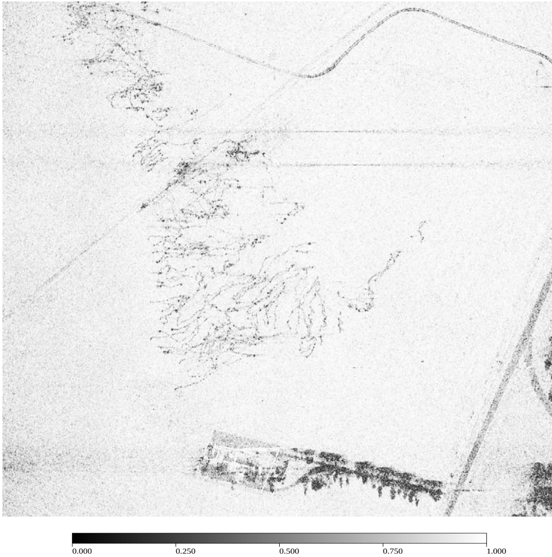
Figure 13: Magnitude image of the sample complex cross correlation coefficient obtained by spatially averaging over a sliding estimation window (2 by 6 pixels in range and azimuth respectively).
