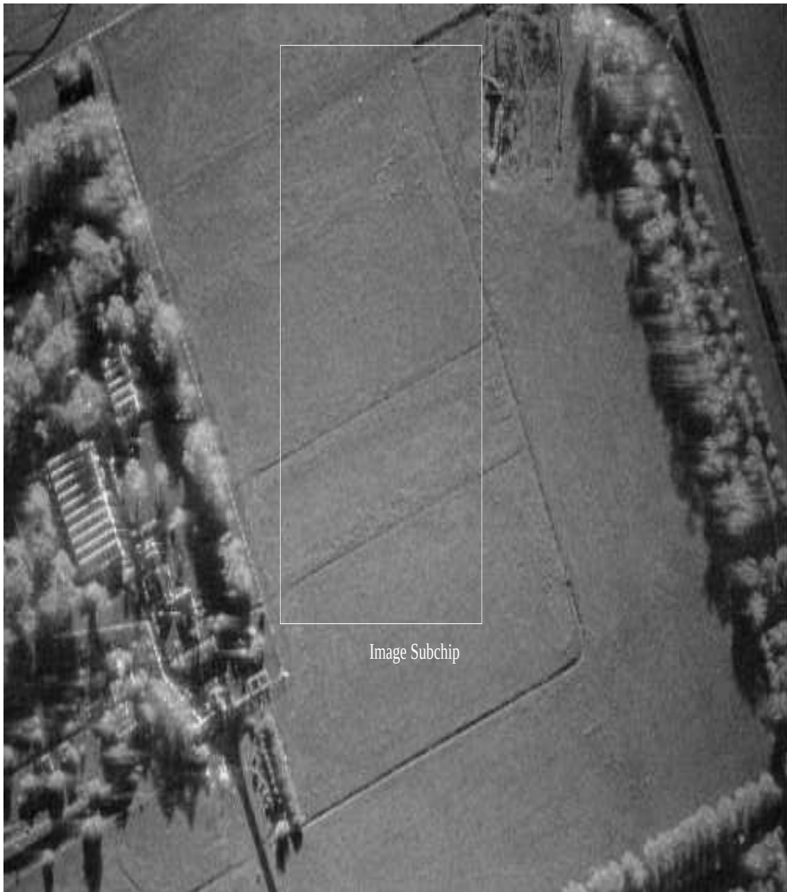
Figure 47: Intensity SAR image generated from the primary pass imaging collection processed to a resolution of 0.52 m (range) by 0.150 m (azimuth) with a Hamming window applied.
