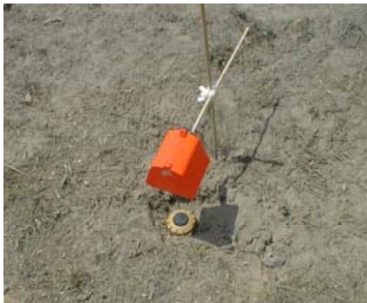
Figure 4: Before and after: Large REMIC-II positioned over a VS-50 AP Landmine, and the completely burned mine after REMIC application.
