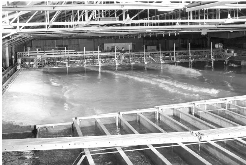
Fig. 1. The LSTF during the plunging case, showing the flow channels (bottom) and the instrument bridge (top) carrying the current meters and wave gages (vertical rods).
