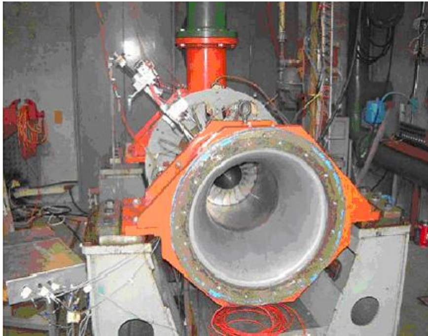
Figure 2. TCR with inlet piping removed [From Ref. 12]
