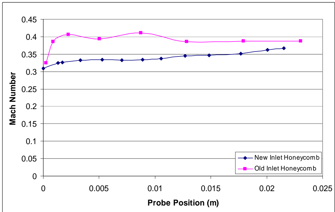
Figure 34. Downstream Mach number distribution at 70% speed, near stall condition
