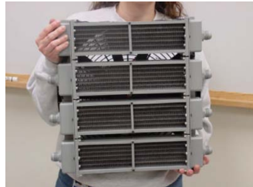
Figure 3: Automotive radiators which demonstrated 33 to 250% performance improvement.
