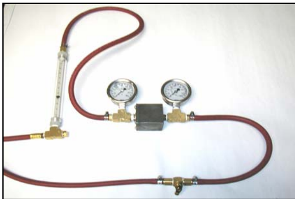
Figure 10: Water and gas flow test apparatus.
