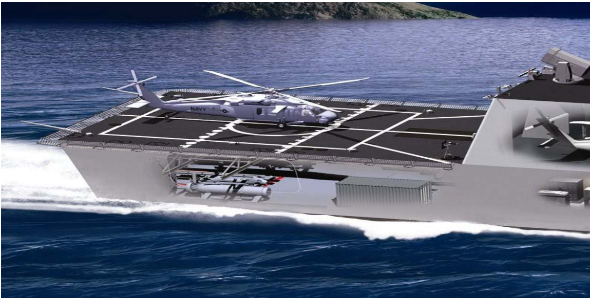
Figure 16. LM LCS Side Door, Launch, Recovery and Handling System, Flight Deck, and Stern Ramp 74
