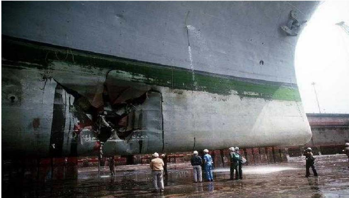
Figure 7. Sea Mine Damage to the USS Tripoli in the Gulf War 25
