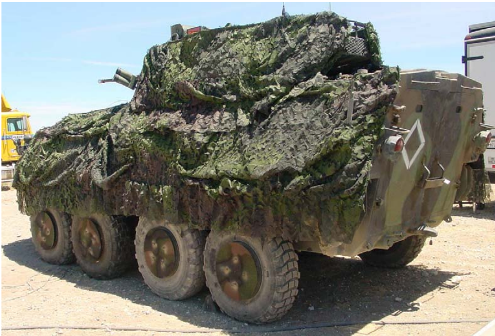
Figure 10 and 11. Depot level camouflage on the LAV-25 consisting of conveyer belt material over the wheels, pieces of ULCANS camouflage netting over the vehicle and with an insulated wooden box over the engine air intake area.
