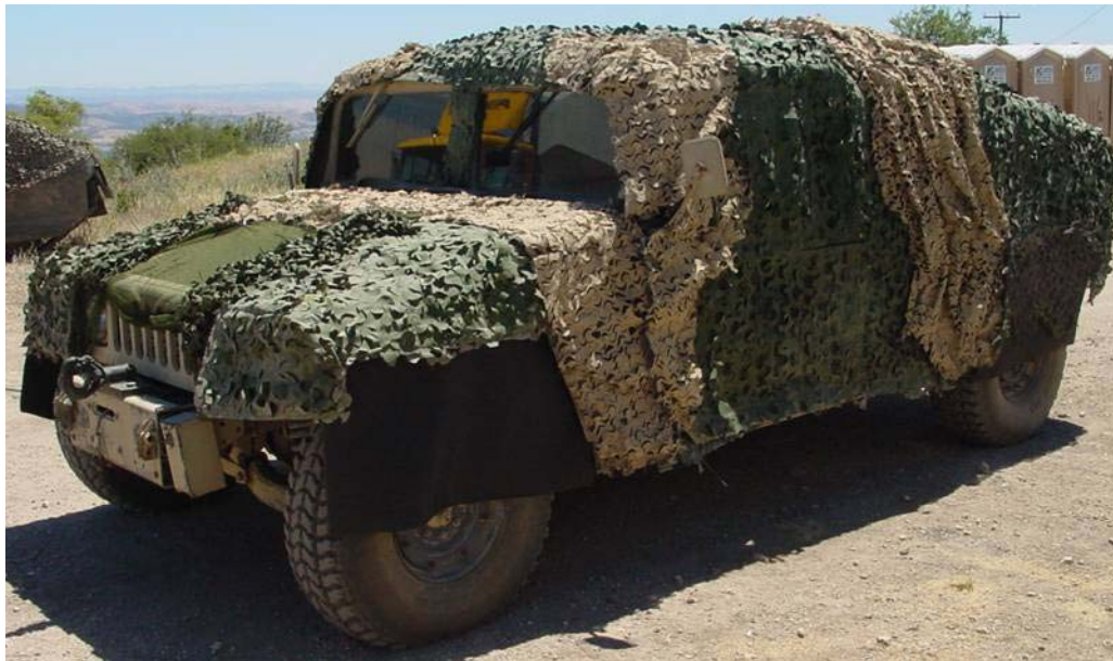
Figure 7 and 8. HMMWV with thermal insulation, camouflage netting, and conveyer belt material
