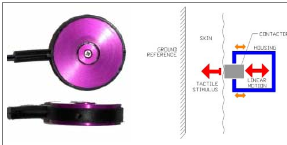
Figure 2. C-2 linear actuator: photograph (left) and operational schematic (right).
