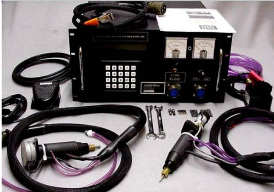
Figure 6. Equipment utilized for ESD repair of components. 1
