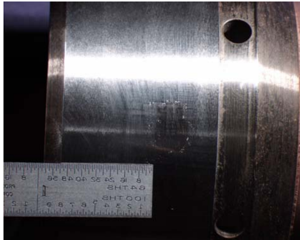
CORROSION PIT AFTER ESD REPAIR AND FINISH GRINDING
