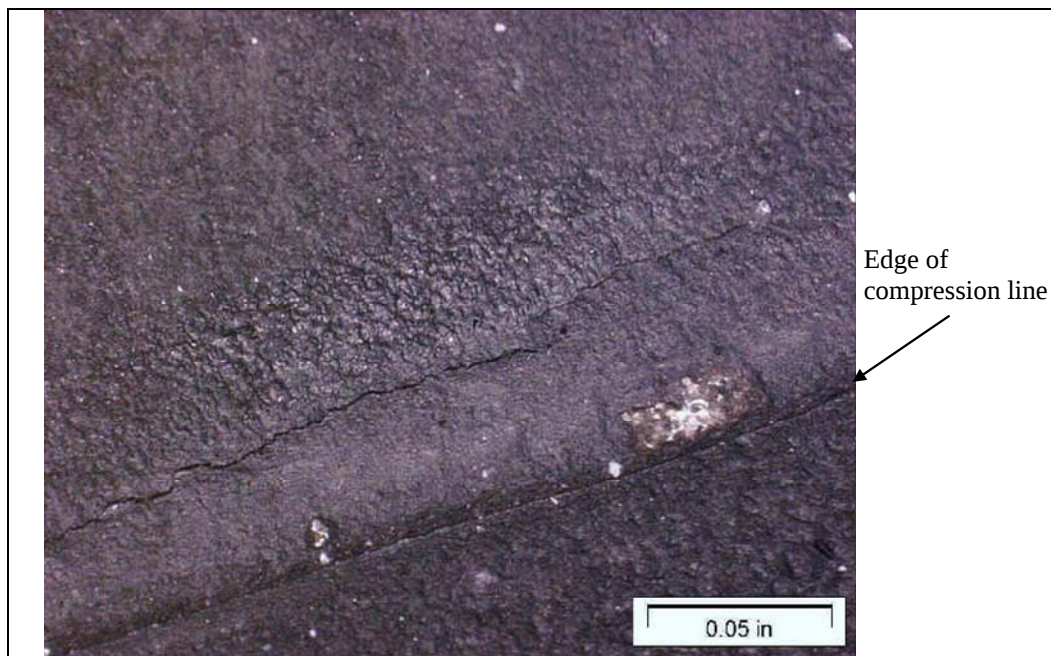
Figure 25. Exterior surface of the tailboom former coated with MIL-P-23377.
