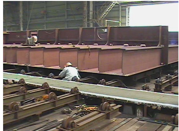
Photo 19: Standard Assembly Method for Double Bottoms
