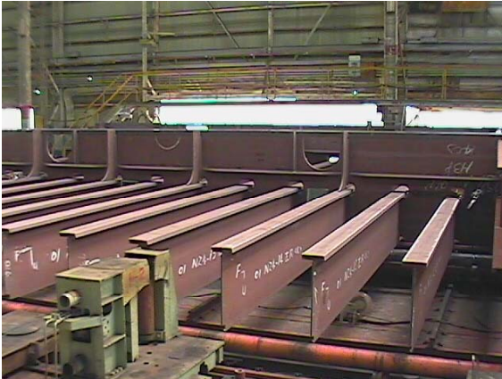
Photo 18: Standard Method for Assembling Webs & Profiles
