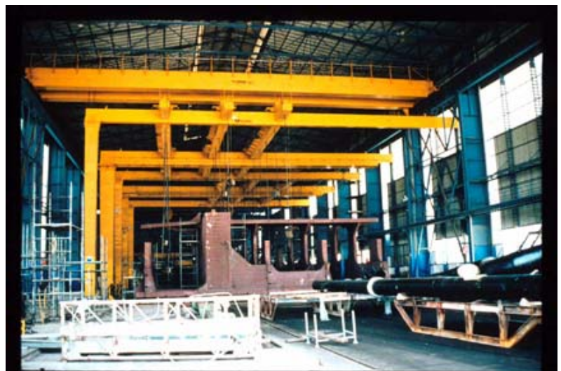
Photo 20: Welding Units Suspended from Overhead
