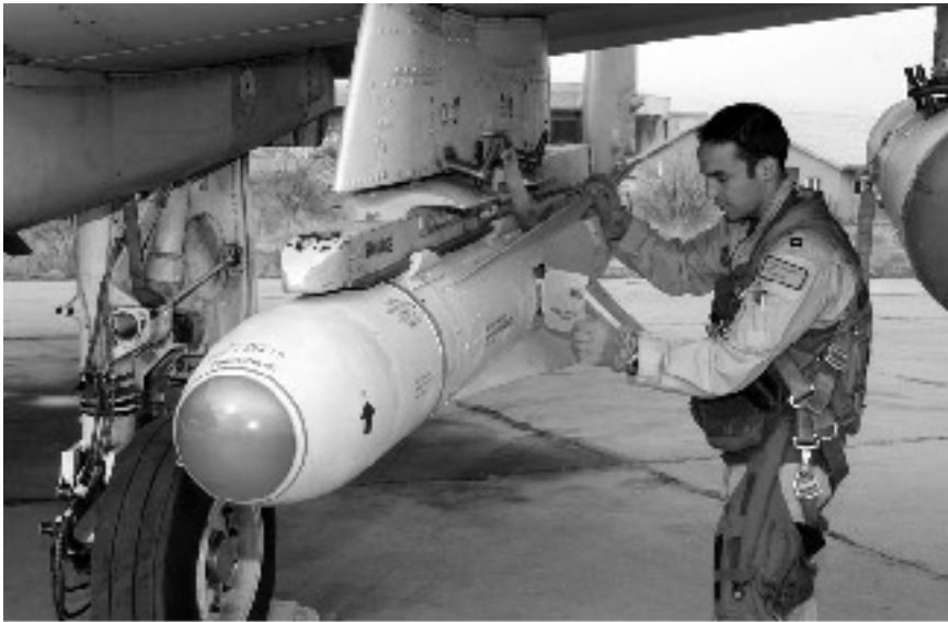
Precision-guided weapon. An A-10 pilot preflights an AGM-65 Maverick air-to-ground missile before launching from a forward-deployed location on a mission to provide CAS for embattled U.S. troops during Operation Anaconda. The imaging infrared sensor installed on the missile allows it to home on both fixed and moving targets with unerringly lethal accuracy.
