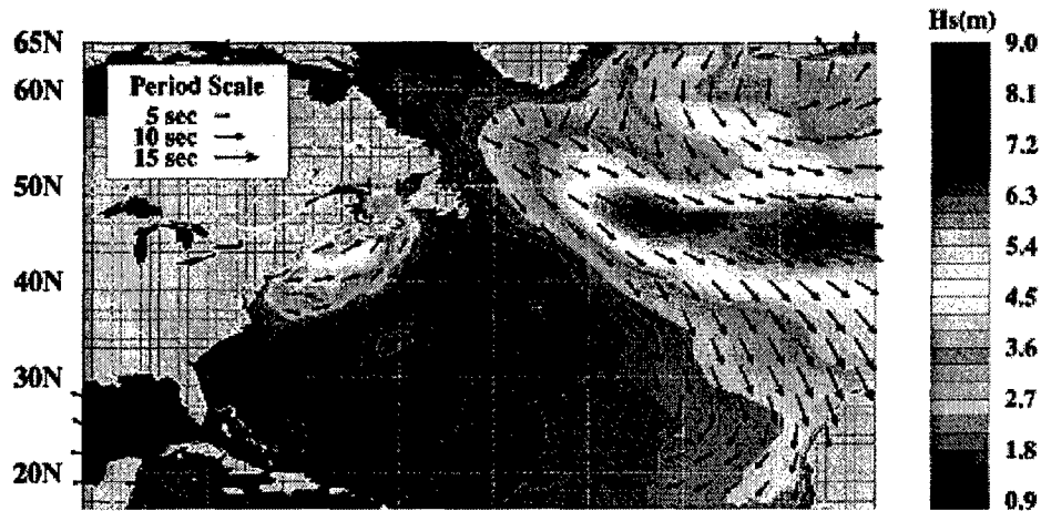
Fig. Wave Heights (contours), Wave Directions (dir. of vectors), Wave Periods (length of vectors) At 2006021800
