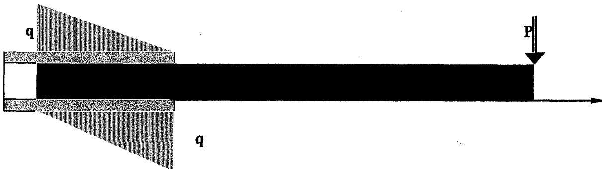
Figure 4.8 Considered Beam Distributed Loading
