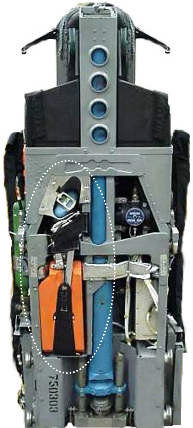
Figure 11. Enhanced Drogue Installation.
