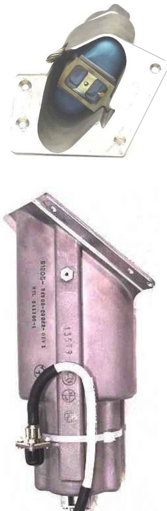
Figure 10. Rocket Installed in Rocket Housing.
