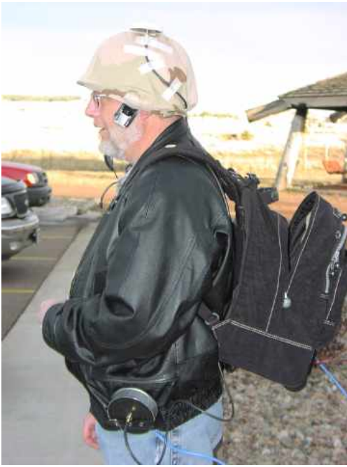
Figure 9 Man-Portable Test Bed Configuration
