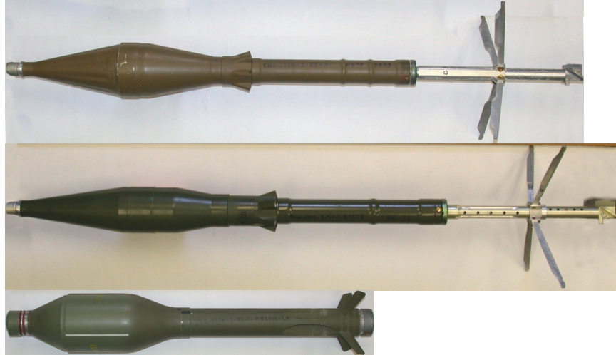
Figure 1. Measured targets: Top, a Chinese Type 69; Middle, a Romanian PG7M; Bottom, a Yugoslavian M57.
