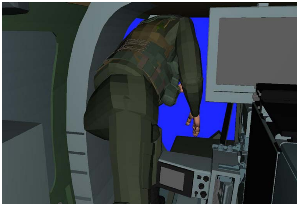
Figure 27. Large male figure leaving through space provided when workstation is folded down.
