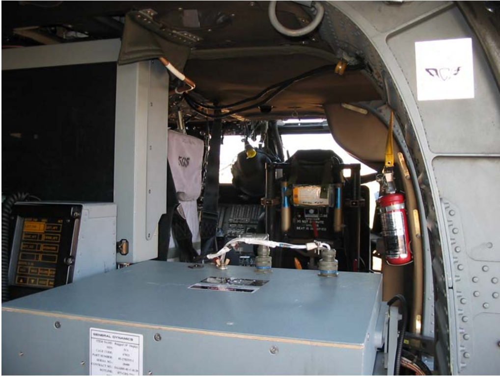
Figure 22. Egress route over workstation.
