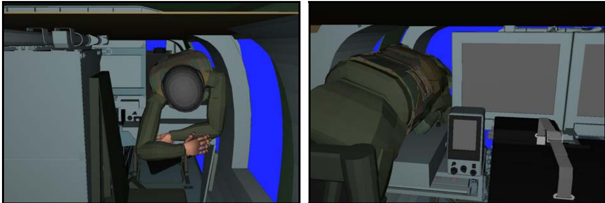
Figure 15. Aft and forward facing views of large male figure clearing shoulders through workstation.
