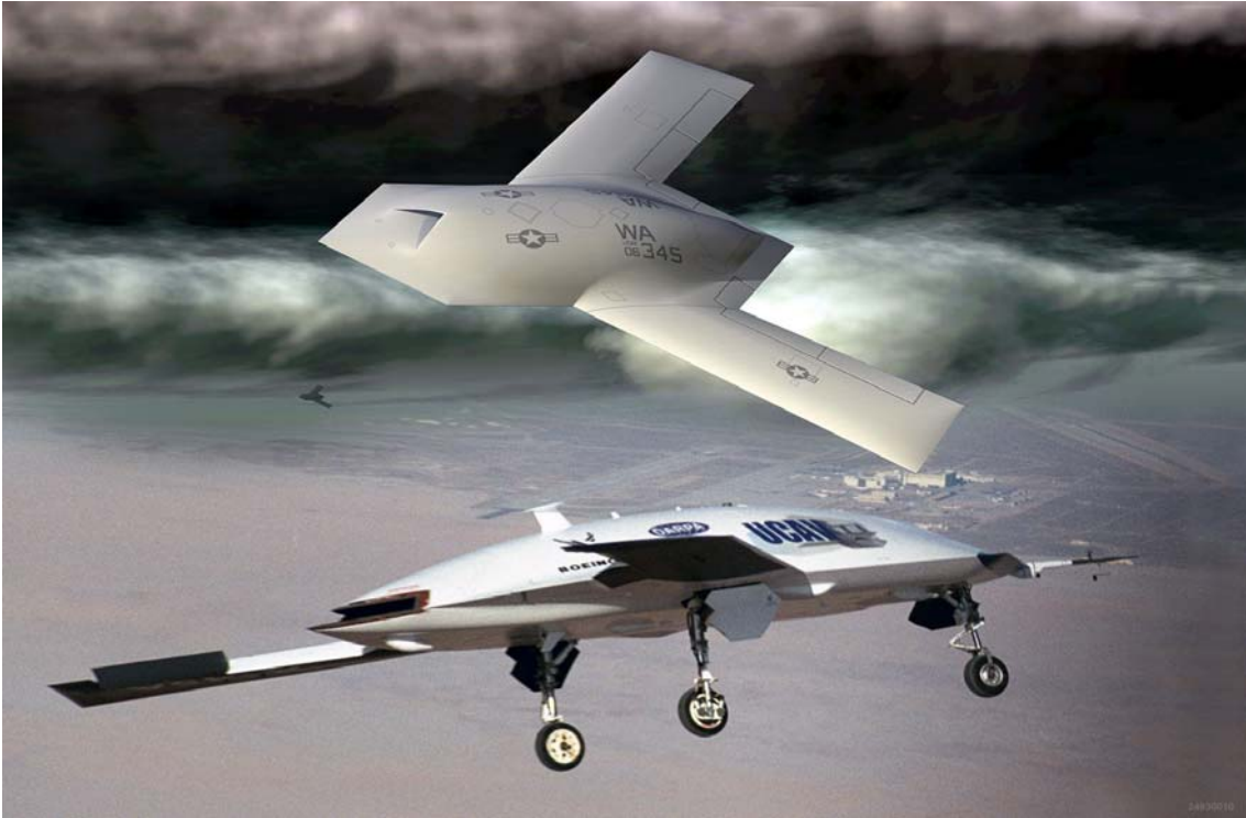
Figure 1. The Boeing X-45A is a UCAV being developed under a joint effort of the Defense Advanced Research Projects Agency (DARPA), the United States Air Force, and the Boeing Phantom Works.
