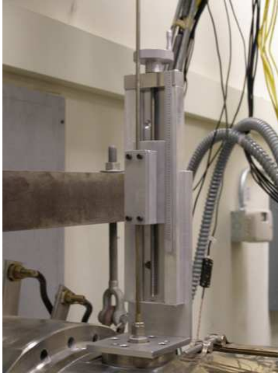
Figure 2.1: Traverse and mount used for contraction measurements
