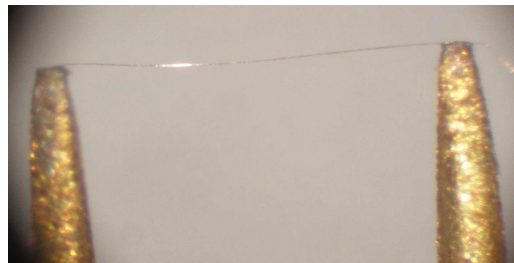
(b) Close up of hot-wire probe tip and wire
