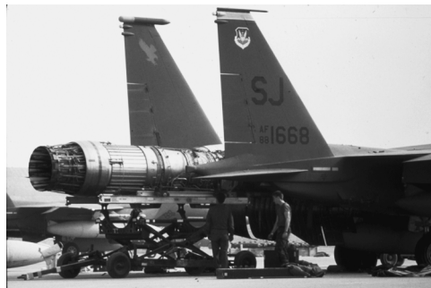
An F-15 receiving an engine change
