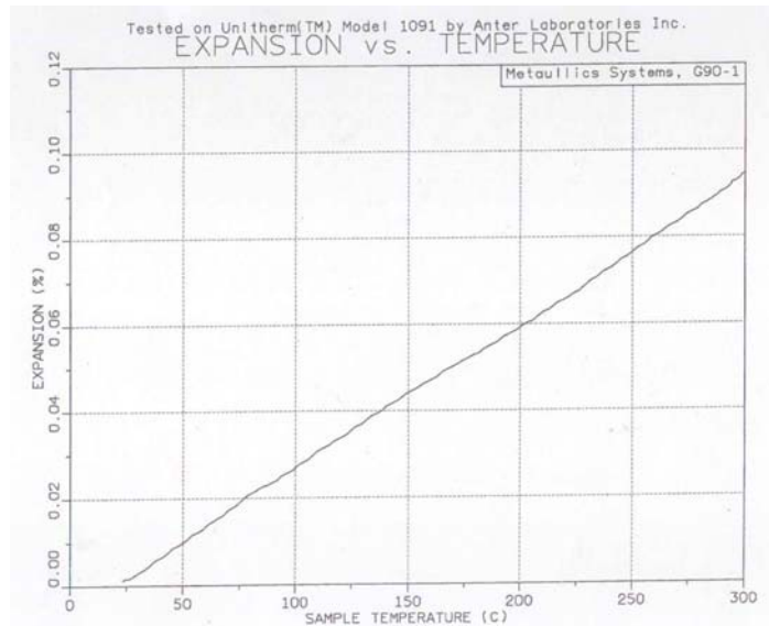
Figure 24. Thermal expansion percentage versus temperature of G-90 graphite.
