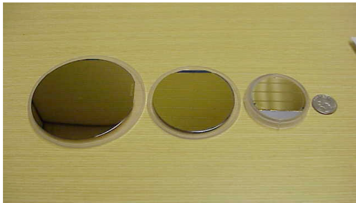
4-in., 3-in., and 2-in. Wafers Shown for Comparison (Compared Against the Size of a Quarter)
