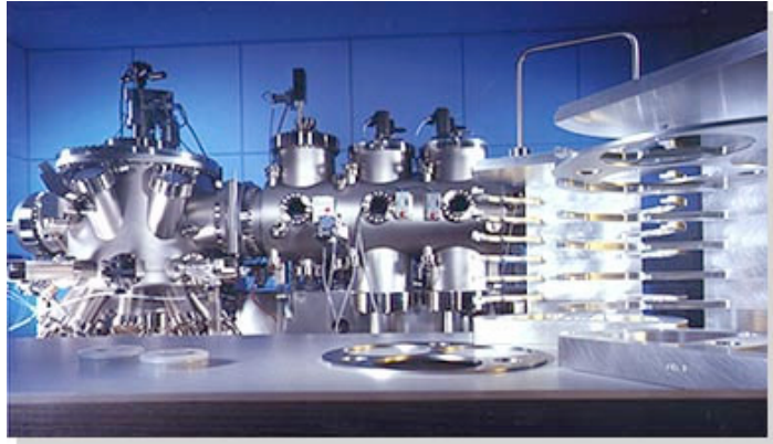
MBE Machine for Fabrication of Laser Diode Wafers
