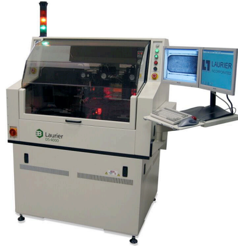
Machine To Stack Bars In Coating Fixtures To Reduce Touch Labor
