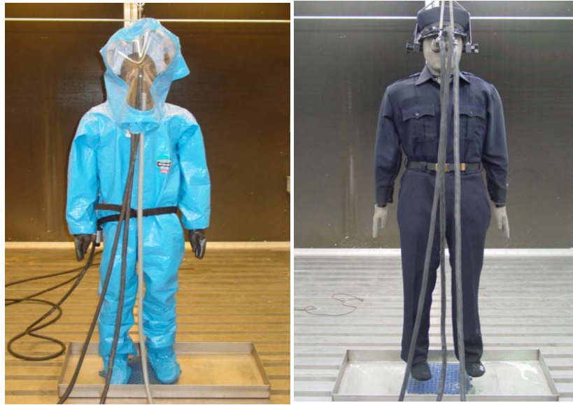
Figure 1. Police Uniform and Level A Uniform on the Thermal Manikin
