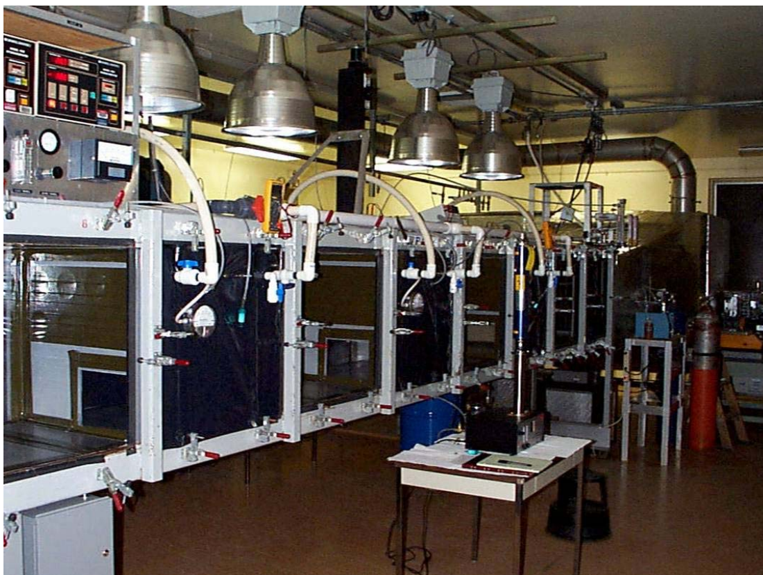
Figure 1. Exposure system used for testing the effects of fog oil and graphite flake aerosols on avian health.
