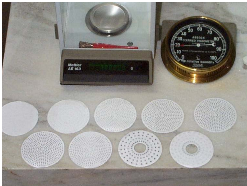
Figure 7. Fog oil and graphite flake aerosol collected on cascade impactor filter inserts.
