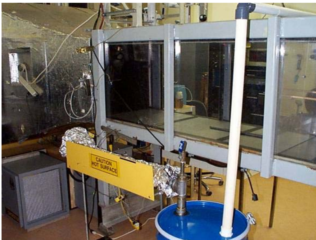
Figure 4. The fog oil generator used to flash vaporize oil which is delivered to a buffer volume (35-gallon drum), then directed as an aerosol to the manifold and test chambers.
