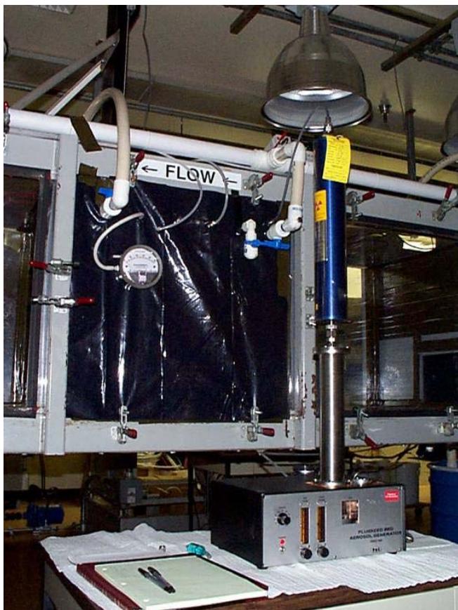
Figure 3. The TSI Model 3400 Fluidized Bed Aerosol Generator used to deliver graphite flake aerosol to the exposure chamber.
