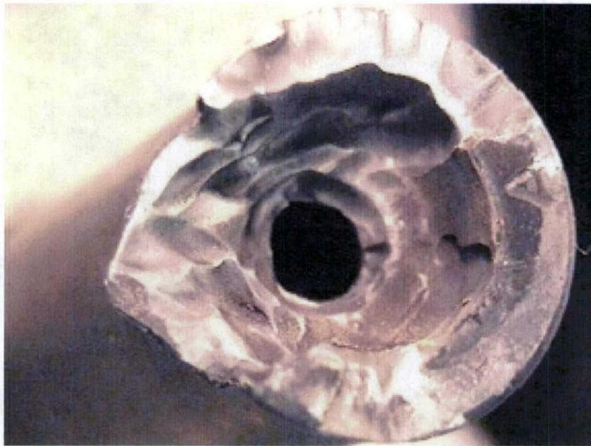
Figure 33 Failed case from hot (+125°F) shot 20, primer area
