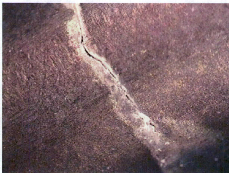
Figure 25 External view of localized case wall split observed
