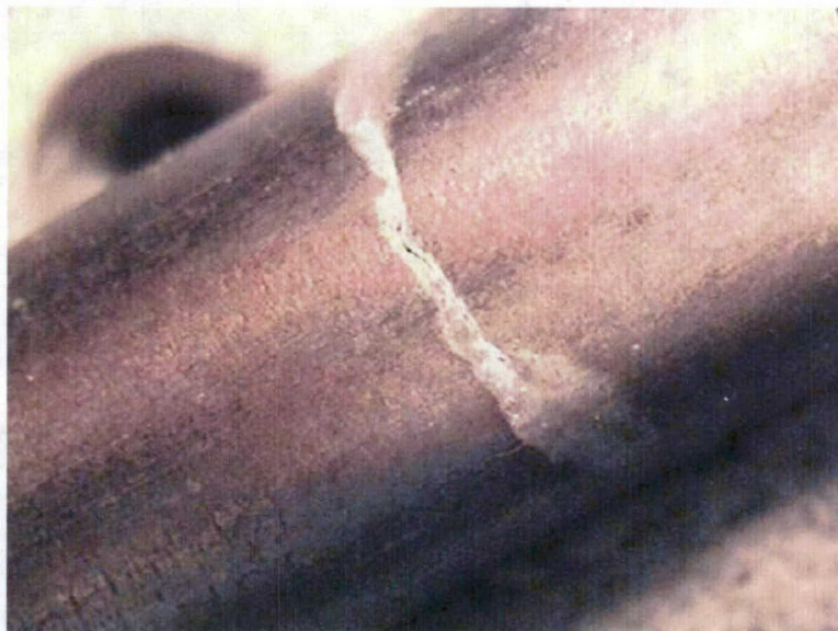
Figure 24 External view of localized case wall split observed
