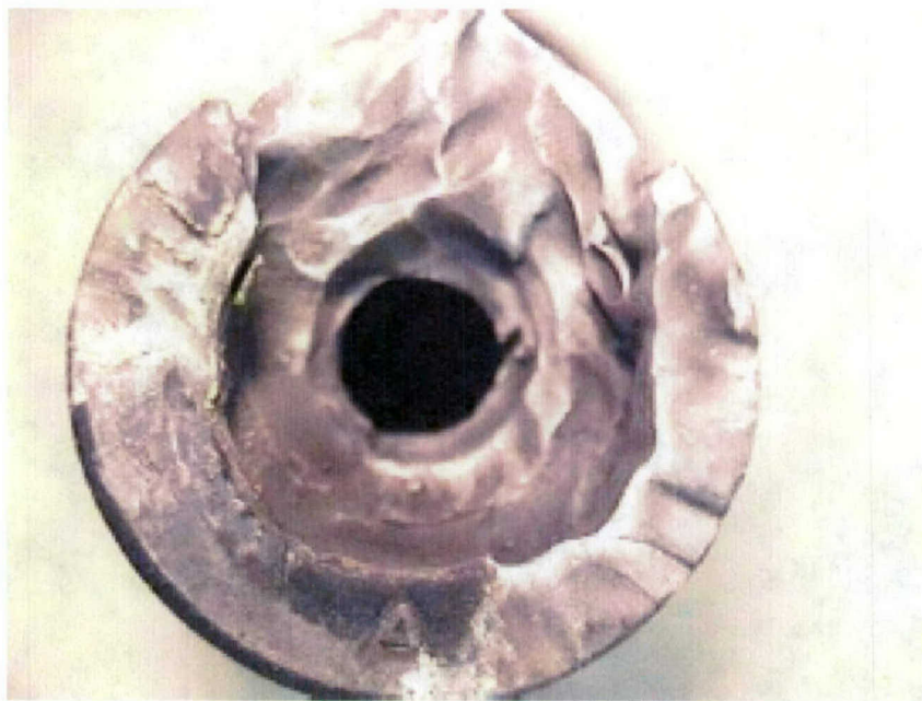
Figure 34 Circumferential failure of case from hot (+125°F) shot 20
