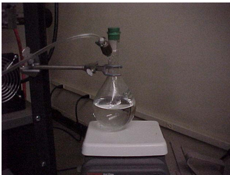
Figure 60. System designed and used to introduce water vapor into the weathering system.
