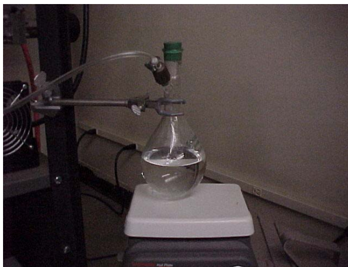
Figure 78. Apparatus used to introduce water vapor into the weathering system.
