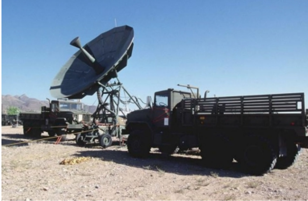
Deployable super-high frequency satellite ground station.
