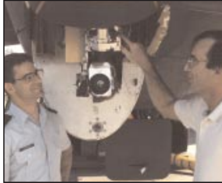
■ Schottky infrared camera mounted on the B-52.
