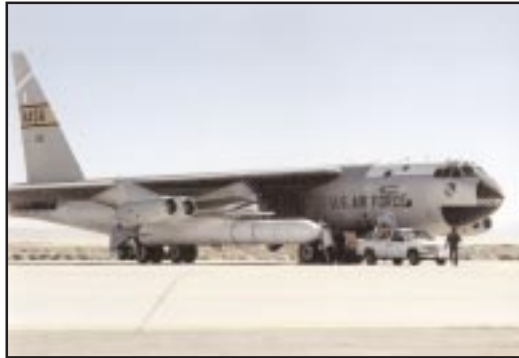
■ Pegasus mounted under B-52 wing.
