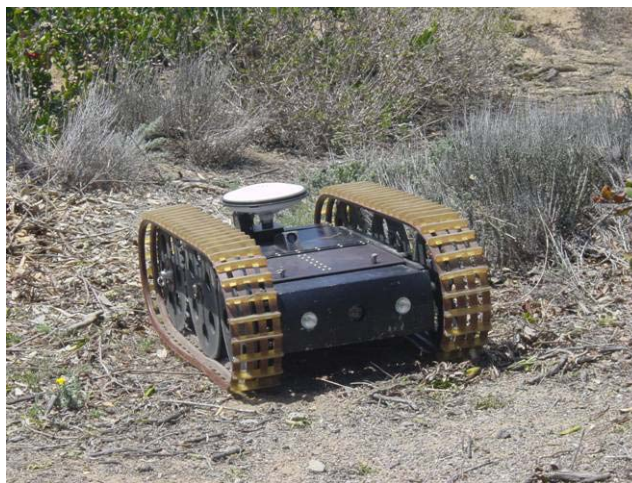
Figure 1. MPRS URBOT w/ GPS Evaluation Antenna
