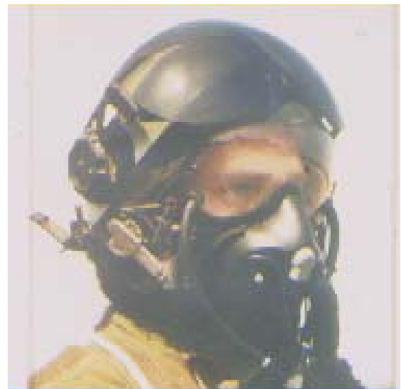
Fig. 33-3. A pilot wearing a Swedish-developed helmet and breathing mask system (mfg by FFV Aerotech AB, Sweden) with chemical-biological protection equipment for use in combination with assisted pressure breathing during acceleration (G). Photograph: FFV Aerotech AB, Sweden.
