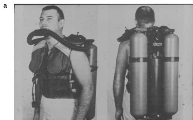
Fig. 31-14. (a) A Mark (Mk) 6 semiclosed-circuit, mixed-gas rebreather. This is a split-bag, recirculating unit, based on a Lambertsen design, which was used by the US Navy from the 1960s through the 1980s. (b) A schematic of the Mk 6 underwater breathing apparatus. Note the similarity of the Mk 6 shown here to the Emerson-Lambertsen closed-circuit oxygen rebreather (see Figure 31-12). The principal difference between the two designs is that the Mk 6 has a relief valve for venting excess gas because nitrogen from the supply gas is not metabolized and collects in the breathing circuit. Photograph a: US Department of the Navy. US Diving Manual . Washington, DC: DN. March 1970: 594. NAVSHIPS 0994-001-9010.
