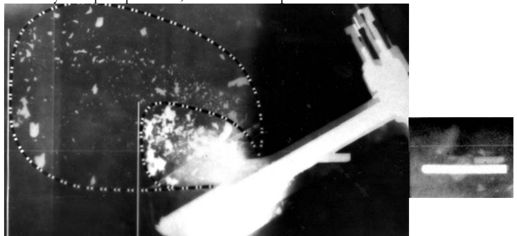
Image of steel rod penetrating steel plate, obtained by flash radiography.
