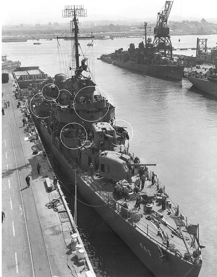
Circles mark recent alterations, including addition of 40mm twin mounts on each side of the forward and midships superstructure
