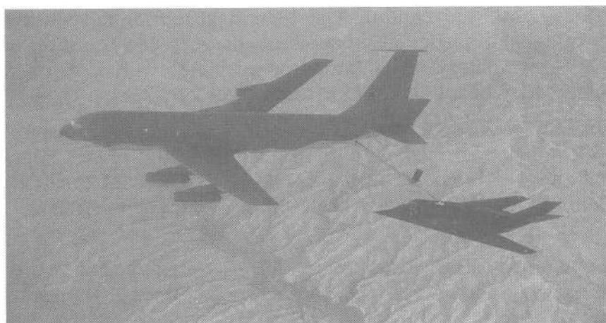
A KC-135 tanker refuels an F-117 Stealth fighter. Designers incorporated radical design and radar-absorbing materials to enable the aircraft to evade radar detection.
