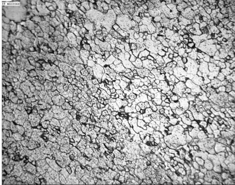
Figure 10. Microstructure of a modified Hipercro 50HS specimen that was cold rolled with deformation slightly more than 3%.
